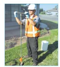
A hand auger is used to bore a hole into the ground.
