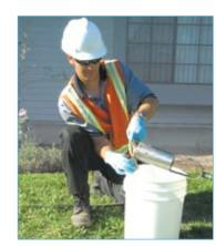
Soil samples are placed in glass sample containers and the containers are stored in a plastic cooler to maintain the integrity of the samples until they are analyzed at an
